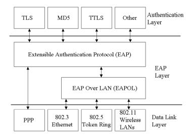
Figure 6: EAP and associated layers
