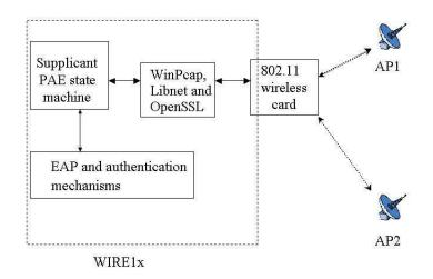
Figure 5: Software architecture of WIRE1x
