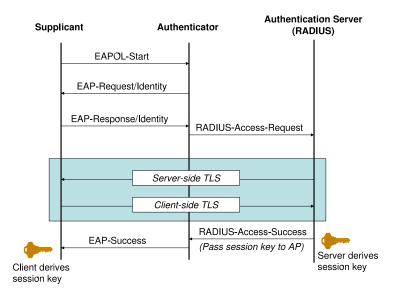
Figure 8: Message flow of EAP-TLS
