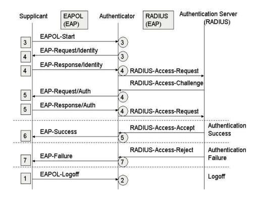
Figure 2: A typical 802.1x message flow
